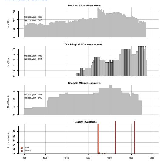
With a total of 191 series, Austria has a very dense glacier monitoring network. FV observations reach back to 1620 and show a relative constant number since 1900. The measurement of MB series started in the 1940s and increased to more than 10 nowadays. A peak in TC records is found around 1980. The glacier inventories have been performed repeatedly, but cover only small parts of the glaciated area.
