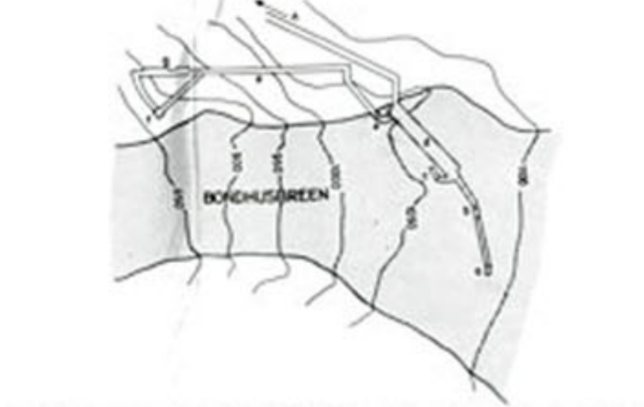
Sketch showing the main subglacial tunnel system: a, b and c are intake shafts, d is the sedimentation chamber, e the unloading tunnel, f the helicopter landing platform, g workshop, h the diverting tunnel leading water to the main reservoir.
